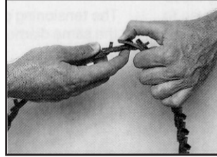
Flex belt further and insert second tab through end link by twisting tab with thumb.
