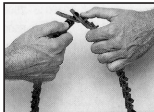
Rotate belt end with tab at 90° to line of belt.
